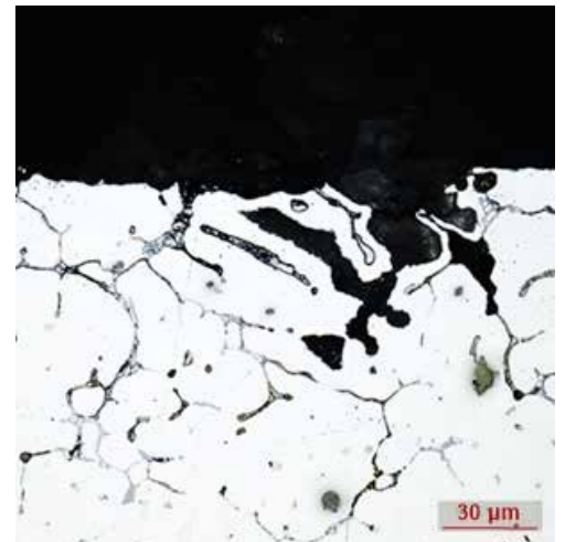
Figure 4: Microstructure of the sample after 480 h in a corrosive environment.
