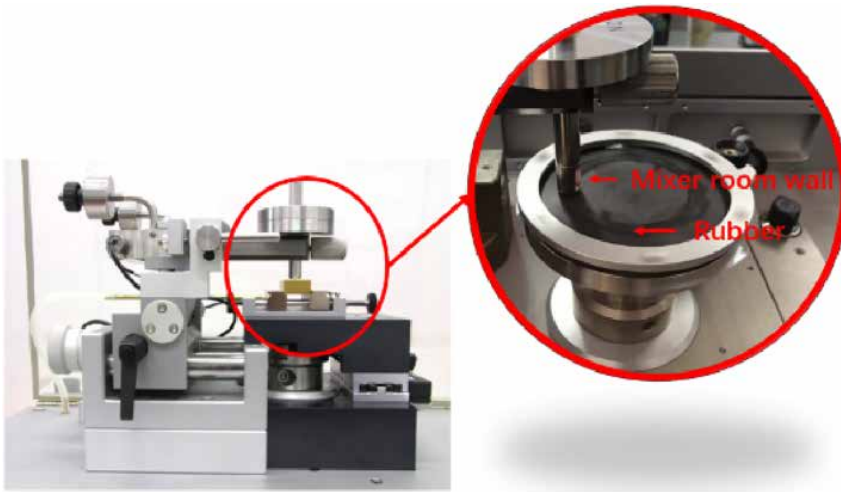
Figure 2: Configuration of the CSM wear test device
